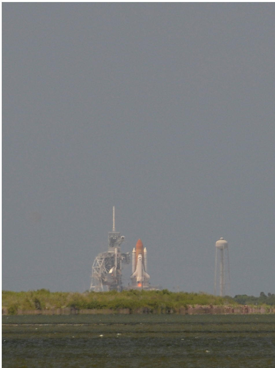
T-5 seconds. Red flame shows up underneath the Shuttle's main engines. They ignite 6.6 seconds before the liftoff.
